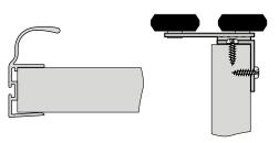
Installation method for angle section Mini 11 mm x 17 mm
