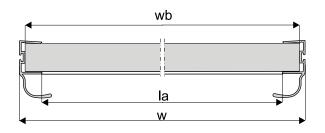
Handle profile should be 2 mm longer than board height. - When fitting handle profiles, do not use assembly adhesive
