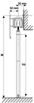
Side fastening of HERAKLES track - max. weight of 80 kg, 120 kg per door
