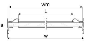
Installation method for fitting 10 mm board (diag. A) and 4 mm mirror or glass (diag. B)
